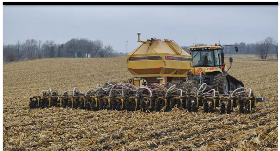
▲ The Soil Warrior’s first pass in the fall tills the top 8-9 in. of soil in a strip while applying fertilizer. The 30-in. cog-wheels and serrated coulters mix fertilizer and residue with the soil. It makes another spring pass using two 20-in. wavy coulters to fluff and condition the top 3-4 in. of soil, adding nitrogen, in strips.
